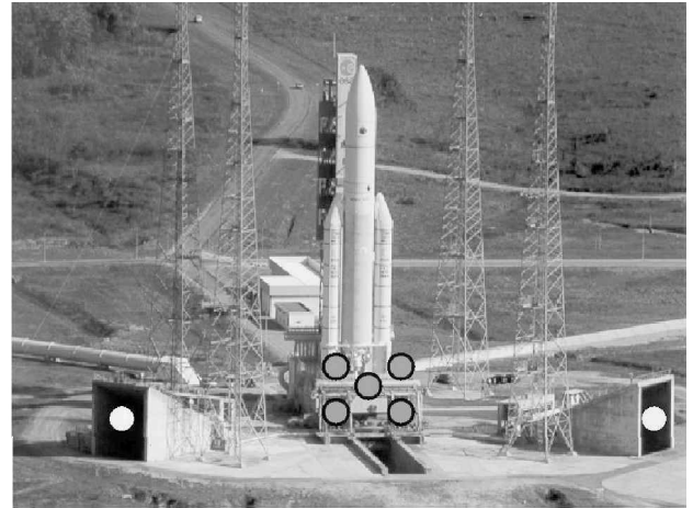
○ EAP Launch Duct Exit Acoustic Sources ● EAP and Vulcain Engine Acoustic Sources
